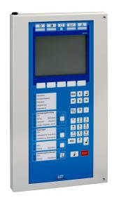
The Remote Display and Operation Panel ABF600-1 is a remote tableau for the operation of a Fire Detection Control Panel BCnet600 and for the indication of its events. It offers the same ease of use and, using LED displays and a graphics display, indicates the same information as a sectional control panel that can be operated.
